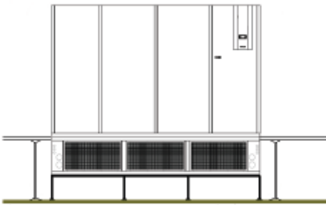
Unit with fan plenum installed under the raised floor
